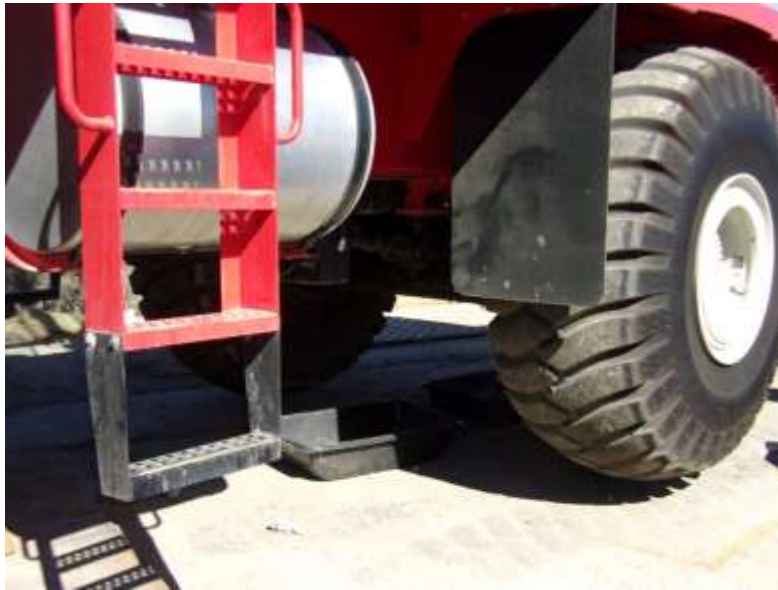
Photo 1: Staged crane at Section 3 bore pit was observed to have a containment bin placed beneath the equipment and spill kits were easily accessible in accordance with MM-HAZ-1a.
